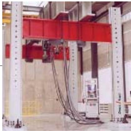
*Large-size test portal for building components and component parts*
