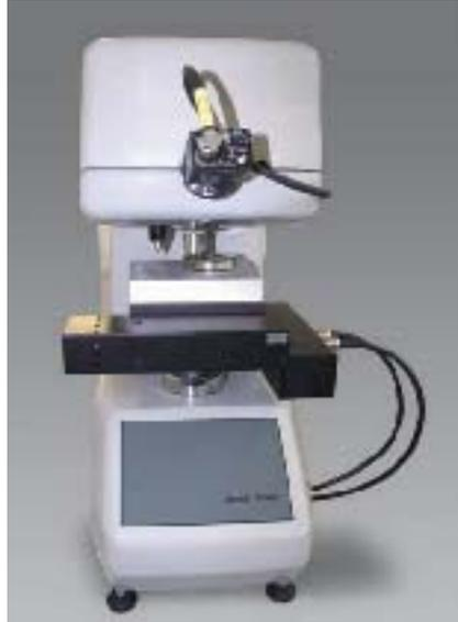
*Zwick / ZHV1 MikroVickers Fully Automatic Hardness Testers*
