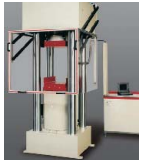
Compression test machine for the testing of building materials, controlled via testXpert® with a vertically adjustable crosshead
