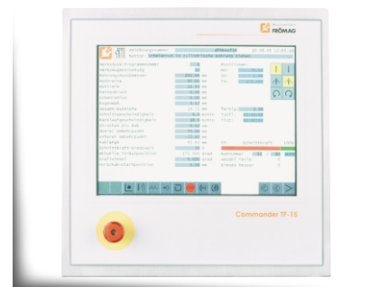
Control panel with 15" touch-screen for CNC
